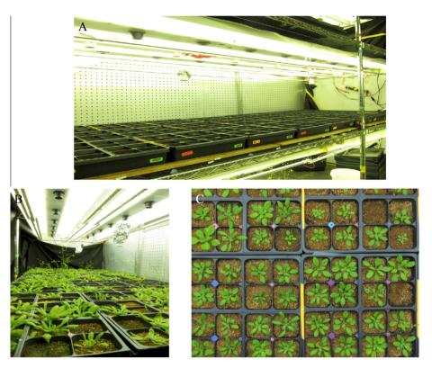
**Fig. 3.** Indoor imaging platform. (A) and (B) show the chamber imaging system on each shelf. (C) is an individual image from one camera. The color-dot system was used to track 4-by-4 pot flat rotation during the growing period. (For interpretation of the references to colour in this figure legend, the reader is referred to the web version of this article.)
